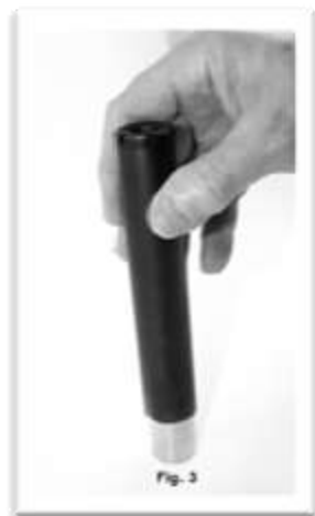
Remove Baffle Stack
